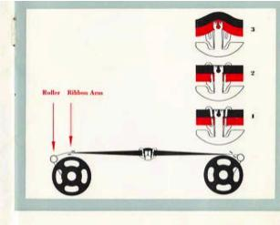
with the finger. Before doing so, move the ribbon arm as far as it will go away from the roller towards the centre of the machine.
