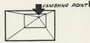
Draw lines from vanishing point to each corner of starting field ..... all fields during a truck in perspective will fall on these lines.
